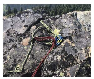
Rappel anchor that failed on Dewey Peak. An investigation concluded the yellow cordelette around the block was held in place by the carabiners linking that cord to a backup cam (not seen). When the backup gear was removed, the cordelette slipped over the block as the last rappeller started down. *Climber 3 Photo*
